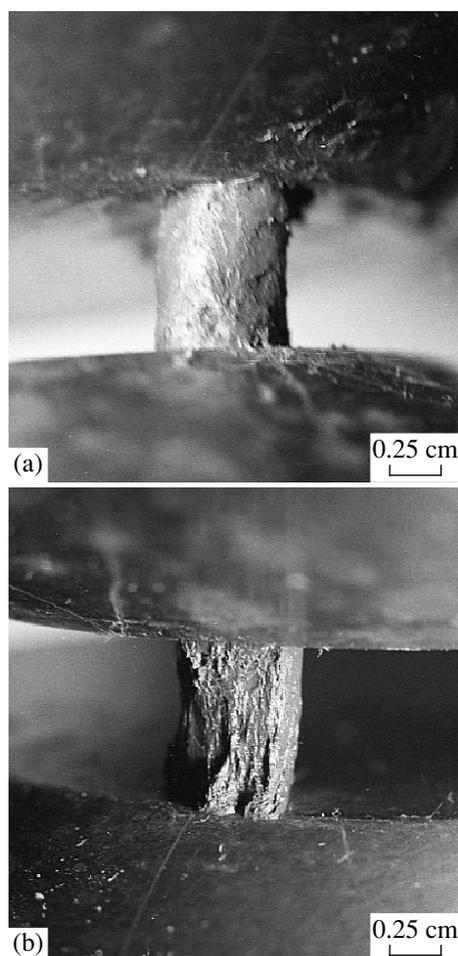
**Fig. 6.** Photographs of the lateral surface of a magnetoelastic sample in uniform magnetic fields of (a) 16 and (b) 557.2 kA/m.
