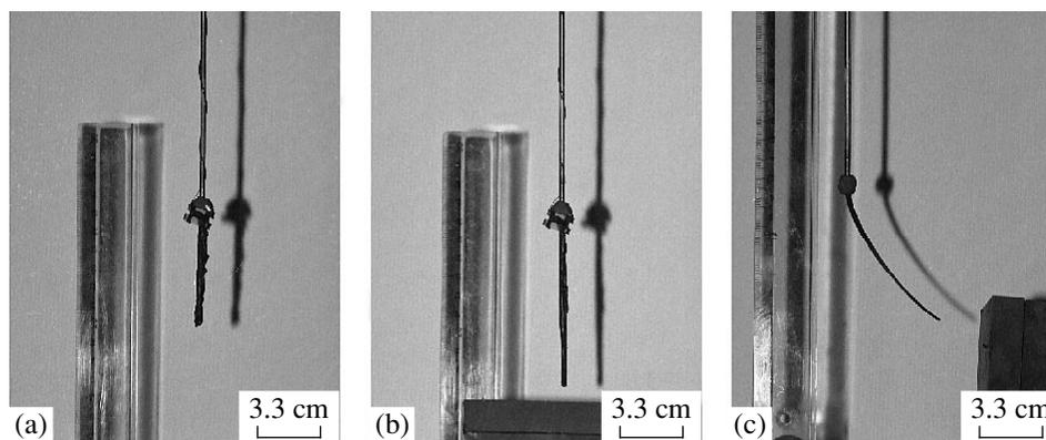
**Fig. 1.** Photographs of a magnetoelastic sample (a) in the absence of field and (b, c) in the field of a permanent magnet.
