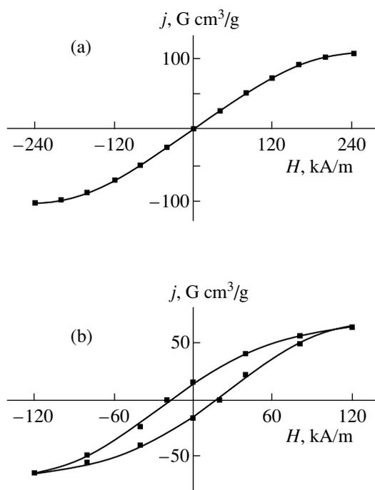
**Fig. 4.** Dependence of the specific magnetization  $j$  on the magnetic field strength  $H$  for magnetoelastics with iron particles of (a)  $2\ \mu\text{m}$  and (b)  $110\ \text{\AA}$  size.
