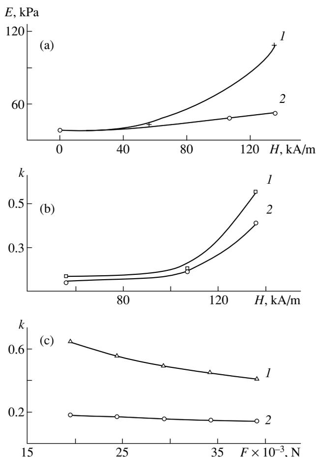
**Fig. 7.** Dependence of (a) the Young moduli (1)  $E_I$  and (2)  $E_{II}$  on the strength of external magnetic field. The volume fraction  $k$  of compressed regions as a function of (b) magnetic field at  $F = (1) 24 \times 10^{-3}$  or (2)  $30 \times 10^{-3} \text{ N}$  and (c) stretching force  $F$  in two different magnetic fields at  $H = (1) 135.3$  and (2)  $58.1 \text{ kA/m}$ .
