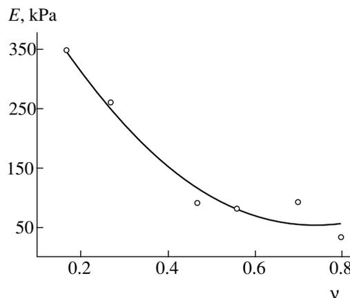
**Fig. 2.** Dependence of the Young modulus  $E$  on the plasticizer mass fraction  $v$  in the polymer matrix for magnetoelastics with the mass fraction of 2- $\mu\text{m}$  iron particles of about 30%.
