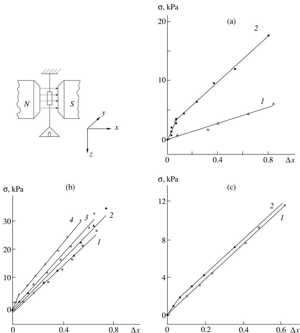
**Fig. 3.** Dependence of the elastic stress  $\sigma$  on the relative elongation  $\Delta x$  for magnetoelastics with the magnetic-phase mass fraction of (a) 42, (b) 30 and (c) 24%, as measured in the absence of field and in different magnetic fields:  $E =$  (a)  $6.9 \times 10^3$ , (b)  $3.8 \times 10^4$ , or (c)  $1.9 \times 10^4$  Pa. The insert shows the scheme of the experiment.
