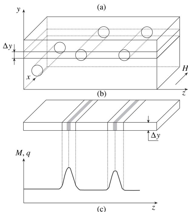
**Fig. 5.** Schematic representation of (a) the structure of a magnetoelastic placed in a uniform magnetic field, with cylindrical contracted regions of the polymer matrix; (b) thin layer of  $\Delta y$  thickness; and (c) magnetization and concentration distributions along the direction  $z$ . The shaded area shows the region with an increased concentration of magnetic particles that is most resistant to stretching.
